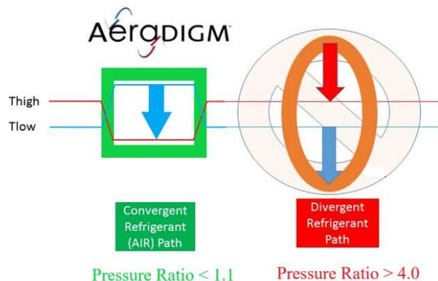
Moreover, the Fan Replacement mechanism which temporarily changes pressure around the heat exchanger also performs the function of a constant pressure heat engine, capturing work otherwise lost in open convection systems as free expansion. No need to burn fuel. Whether cooling or heating, the work produced by adiabatic expansion or contraction depends only on the change in temperature and the heat capacity of the gas.
