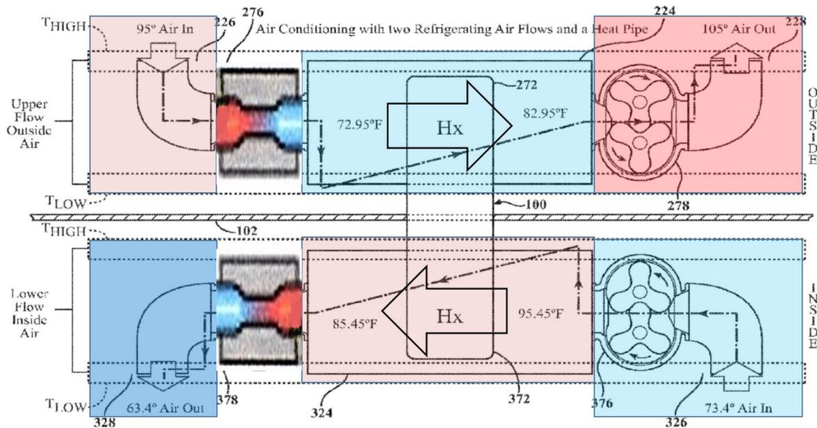
3. By replacing the sonic nozzle with a companion pump to manage the pressure across the heat exchanger, the work of compression will be directly recovered, increasing the overall energy reduction to 75% as previously outlined. (All components well proven in commercial use since 1965. Patents pending.)
