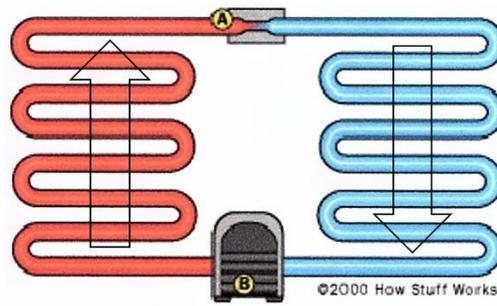
The blue (cool) flow is in the low-pressure zone, from the sonic nozzle to the compressor.
